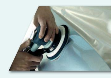
Norgrip® and Soft-Touch® discs have a quick release backing that allows quick and easy disc changing, increasing performance by minimising downtime. Soft-Touch® discs also include a foam backing that improves product performance and gives an even longer product life. The foam layer absorbs unevenness in the surface, helping to maintain an excellent cutting action providing a very homogenous, high quality finish.
