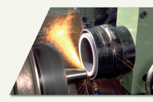
Cylinders are relatively soft and have a thin contact area. They are normally used in a chuck or fixed to a plate. The part is held on a table and either reciprocates or turns in a clockwise direction. To improve safety, cylinders are bound with layers of multi-filament high strength tape.
